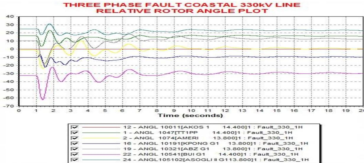
**Figure 16:** Case 1 – Speed of machines on the grid for 330kV three phase fault
