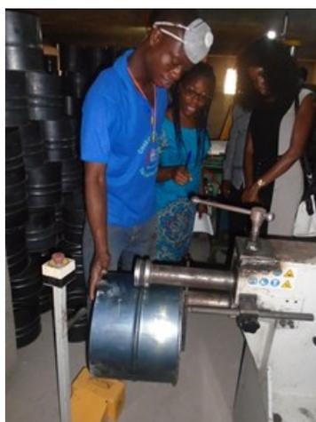
Rolling of stove (top); Cutting of Combustion Chamber (bottom left) followed by Punching of Holes for Chamber (right)
