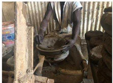
Photo Above: Artisan Moulding a Liner with Clay
