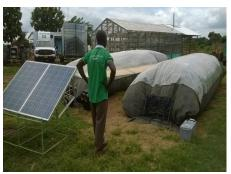
Solar-Gas Hybrid Mobile Dryer (above) and Solar Biomass Hybrid Dryer (below) developed by PENS Food Bank
