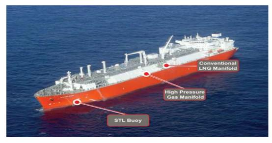
Figure A3. LNG Energy Bridge Regasification Vessel
