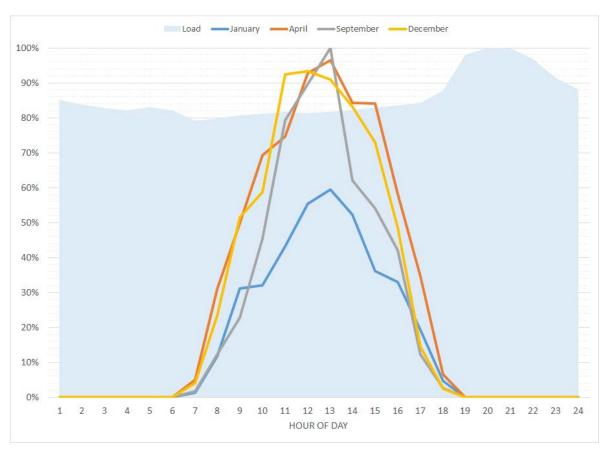
Figure ES-1: Normalized Ghana System Load and Normalized Average Monthly Solar PV Output
