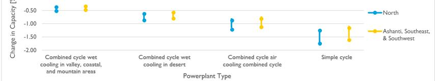
Figure 24. Potential change in natural gas fired power plant capacity based on change in average annual temperature for the North and for Ashanti, the Southeast, and the Southwest regions. The upper bound represents the change in capacity associated with RCP 4.5 projections, while the lower bound represents change in capacity associated with RCP 8.5 projections. Capacity-temperature relationship based on Sathaye et al. 2013, Neumann and Price 2009, and Acclimatise 2009.
