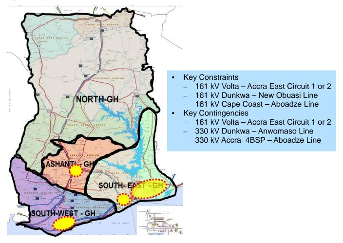
The results of the export capability assessment from the Akosombo/Kpong/Tema generation center to the rest of the GRIDCo system is shown in Table 10. The firm and non-firm export capabilities are 451 MW and 1,099 MW respectively. In both cases the transfers are limited by the double circuit 161 kV Volta to Accra East line. Firm exports are limited to 451 MW by one
