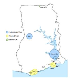
Figure 20. Ghana generation plants, where circle size is proportional to capacity. Source: Modified from Power Systems Energy Consulting (PSEC) and Ghana Grid Company Limited (GRIDCo) 2010 Ghana Wholesale Power Reliability Assessment.
