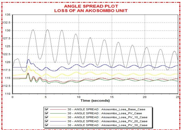
Figure 8: Rotor Angle Plot Showing Impact of Loss of an Akosombo Hydroelectric Unit
