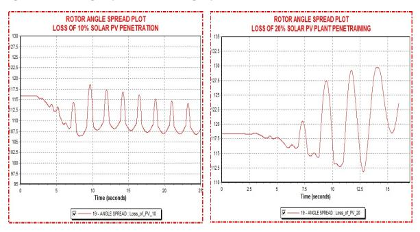
Figure 13: Rotor Angle Spread Plot Showing Impact of Loss of Solar PV Generation
