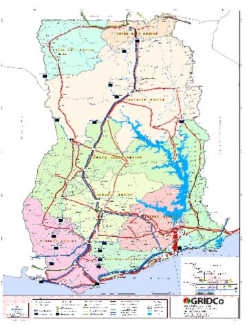
Figure 26. Ghana existing (solid lines) and planned (hashed lines) transmission and distribution system. Lines range from 330 kV (blue), 225 kV (green), 161 kV (red and yellow), and 69 kV (black). White squares represent existing substations.
