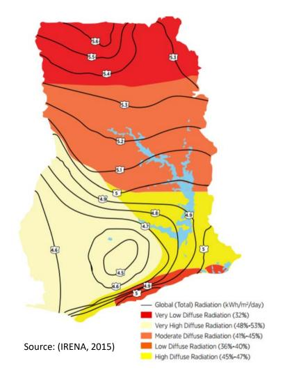
Figure 4: Global Solar Irradiation in Ghana
