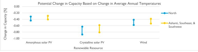
Figure 25. Potential change in solar PV and wind capacity based on change in average annual temperature for the North and for Ashanti, the Southeast, and the Southwest regions for 2040-2059 relative to the historical period 1986-2015. The upper bound represents the change in capacity associated with RCP 4.5 projections, while the lower bound represents change in capacity associated with RCP 8.5 projections. Capacity-temperature relationship based on ADB 2012 and Solar Facts n.d.
