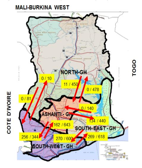
Figure 4: Ghana Bulk Power System Transfer Capability – 2018
