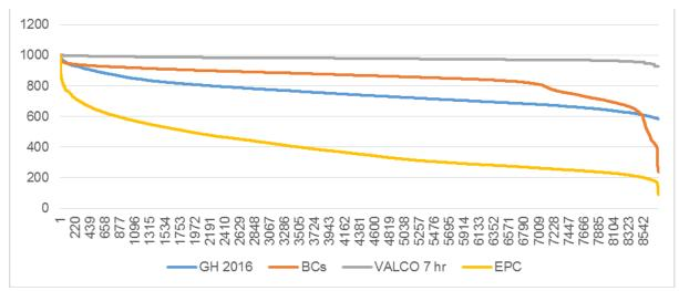
Figure 26: Load Duration Curves scaled to a 1000 MW Peak
